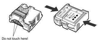
**5.** After removing the partially used BJ Cartridge, use the BJ Cartridge Container SB-10 supplied with the printer.
